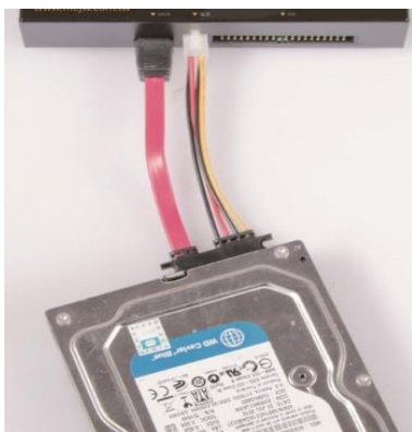
Connect SATA HDD/SSD
