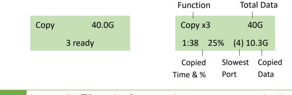
Press "▲ ▼" together for 5 seconds to stop operation on the slowest device.
